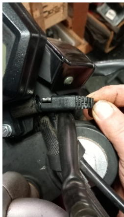
Replace the croc clips with eyelets
